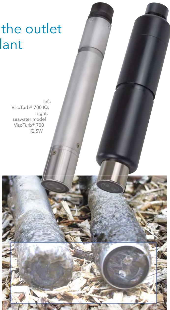
Sensor without and with ultrasound cleaning system after 30 days
